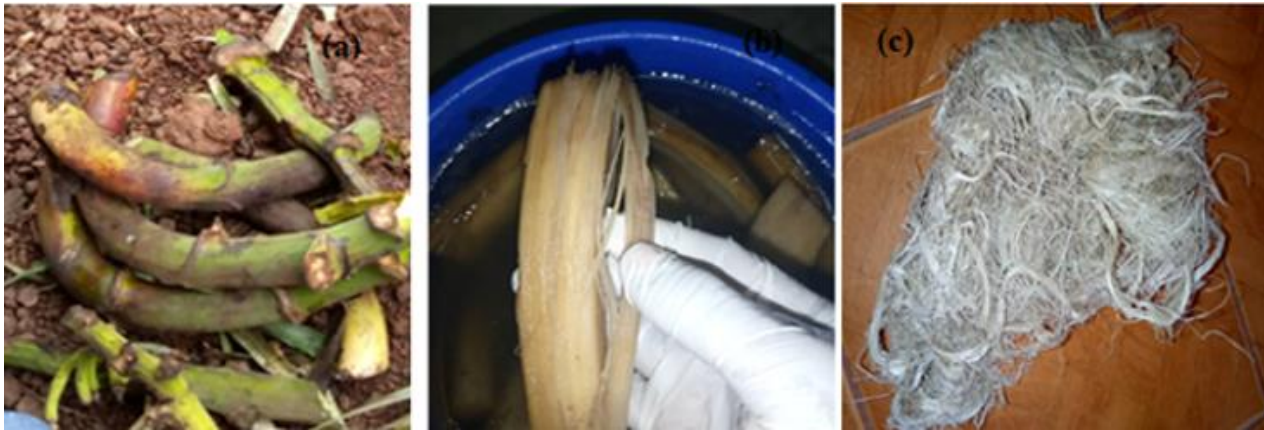
Fig.1. Retting process of banana stalk fiber. (a) Longitudinal view of raw banana tree stalk, (b) Banana tree stalk in distilled water, (c) Extracted fibers.
