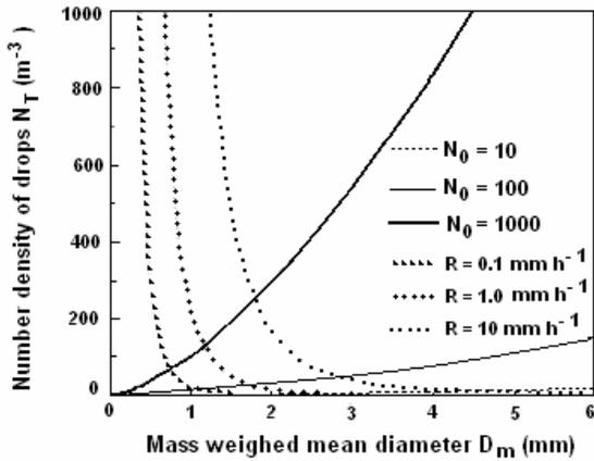
Fig. 3.  $N_T - D_m$  for different  $N_0$  and  $R$  at constant  $\mu$  according to eq. (21) and eq. (15) respectively.
