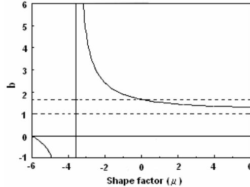
Fig. 1. Dependence of  $b$  on DSD shape parameter considering exponent of (3) as 0.67.  $b$  is the power of ( $Z$ - $R$ ) relation.
