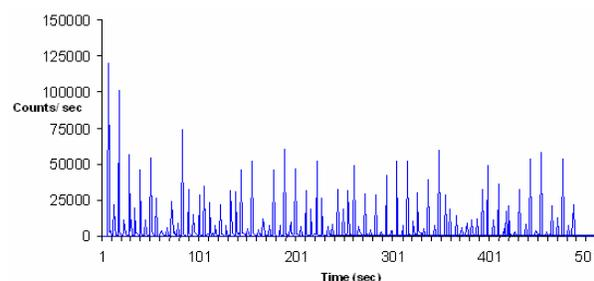
Fig. 4. Time spectrum of a sample corresponding to a completely degraded area on the sample. This is clear from the time taken to reach the substrate, which is about 2 seconds.
