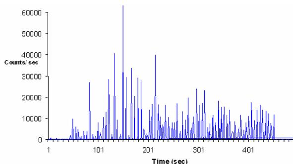
Fig. 6. Time-spectrum corresponding to a coated steel sample where the protective coating was considerably attenuated. The time taken for the laser to reach the substrate was about 45 seconds.
