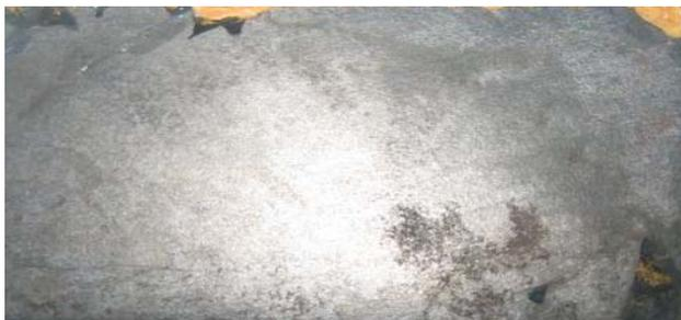
Fig. 1. Coated steel sample showing early stages of degradation.
