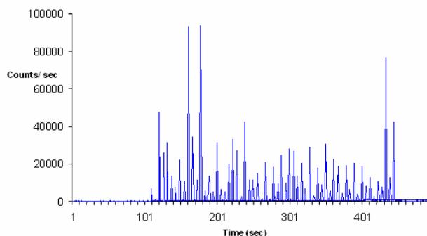
Fig. 5. Time spectrum of a coated steel sample where the protective coating is weakening. This is evident from the shorter time taken to reach the substrate - just over 100 seconds.
