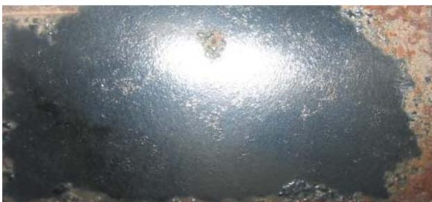
Fig. 2. Coated steel sample showing advanced deterioration around some edges.
