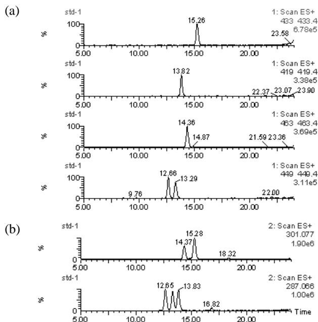
Fig. 5. Extracted ion chromatograms of anthocyanin standards (a) low cone voltage MS data (b) high cone voltage MS data.
