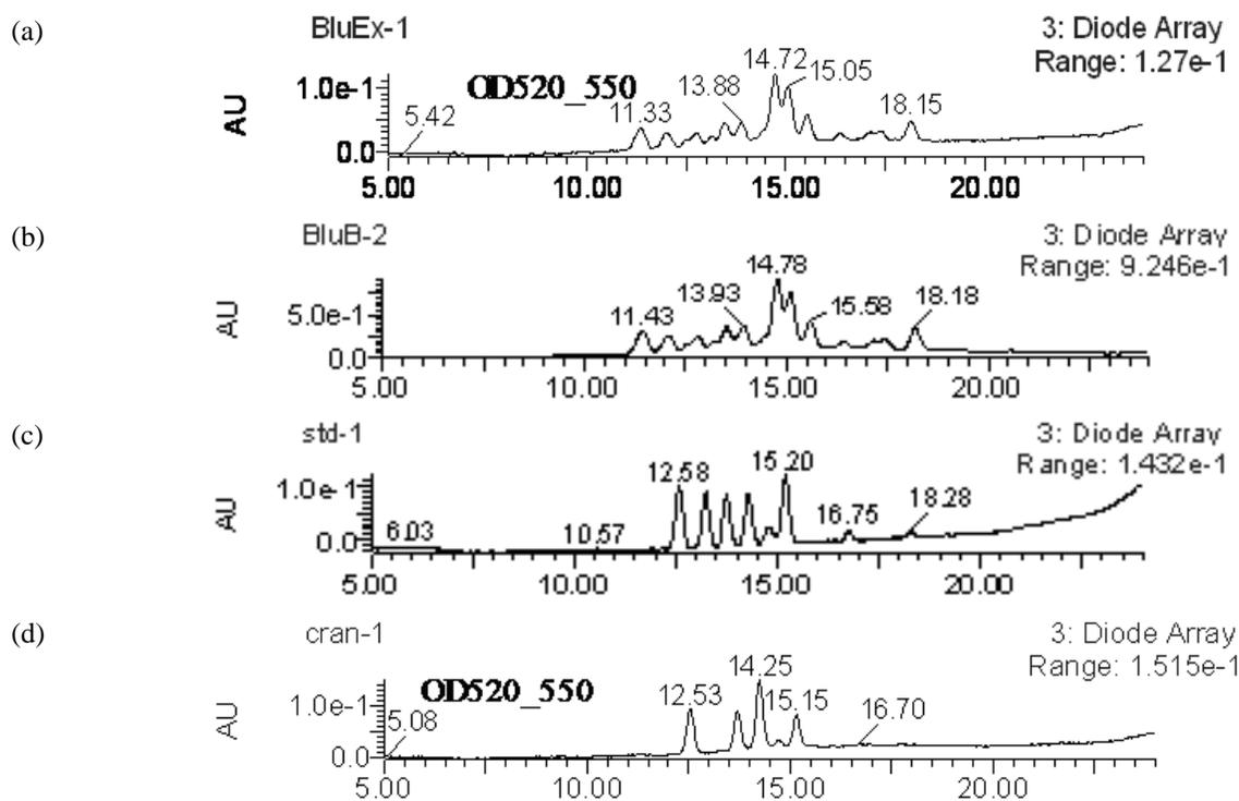
Fig. 4. HPLC chromatograms for (a) Blueberry extract (b) Blueberry juice with 10-fold dilution (c) Anthocyanin standards (see Experimental for concentrations), and (d) Cranberry juice; all monitored at a wavelength of 520 nm.
