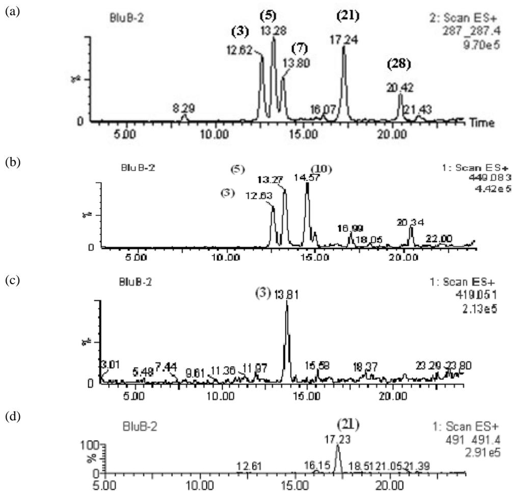
Fig. 6. LC-MS data of blueberry juice. (a) MS data of fragments with  $m/z=287$  showing cyanidin-containing compounds. (b) MS data of compounds 3, 5, 10 that have  $MW = 449$  cyanidin 3-galactoside, cyanidin 3-glucoside, and petunidin 3-arabinoside. (c) MS data of compound 7 that has  $MW$  of 419, cyanidin 3-arabinoside (d) MS data of compound 21 that has  $MW$  of 491, cyanidin 3-acetylated glucoside.
