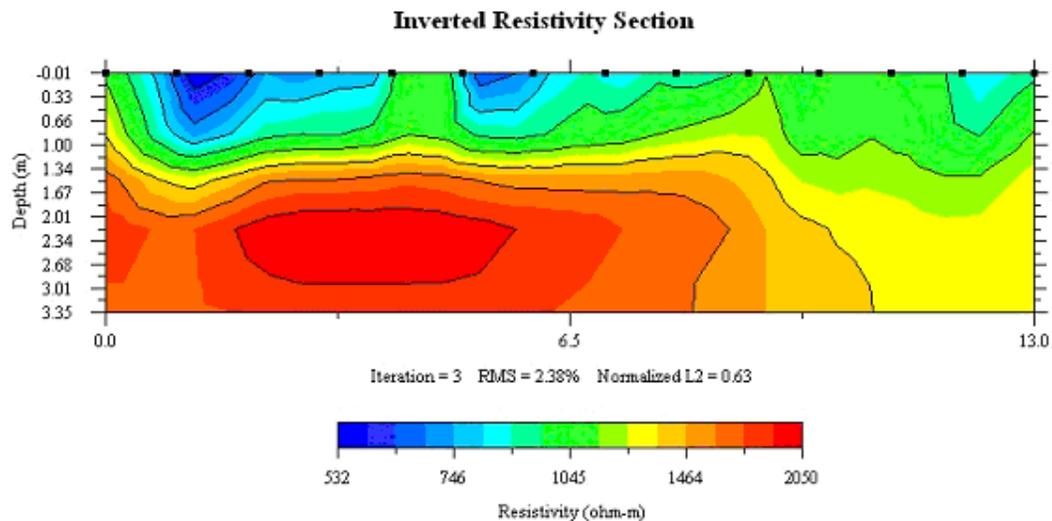
Fig. 2. Electrical resistance cross section from lateral moraine. Upslope is to the right of the figure. Moderate resistance near on the upper slopes indicates dry, unconsolidated glacial materials. Low resistance near the surface on the downslope end of the section (the left side of the figure) indicates water in the glacial material. The high resistance area that occurs at approximately 1.5 meters beneath the surface indicates discontinuous ice lenses.
