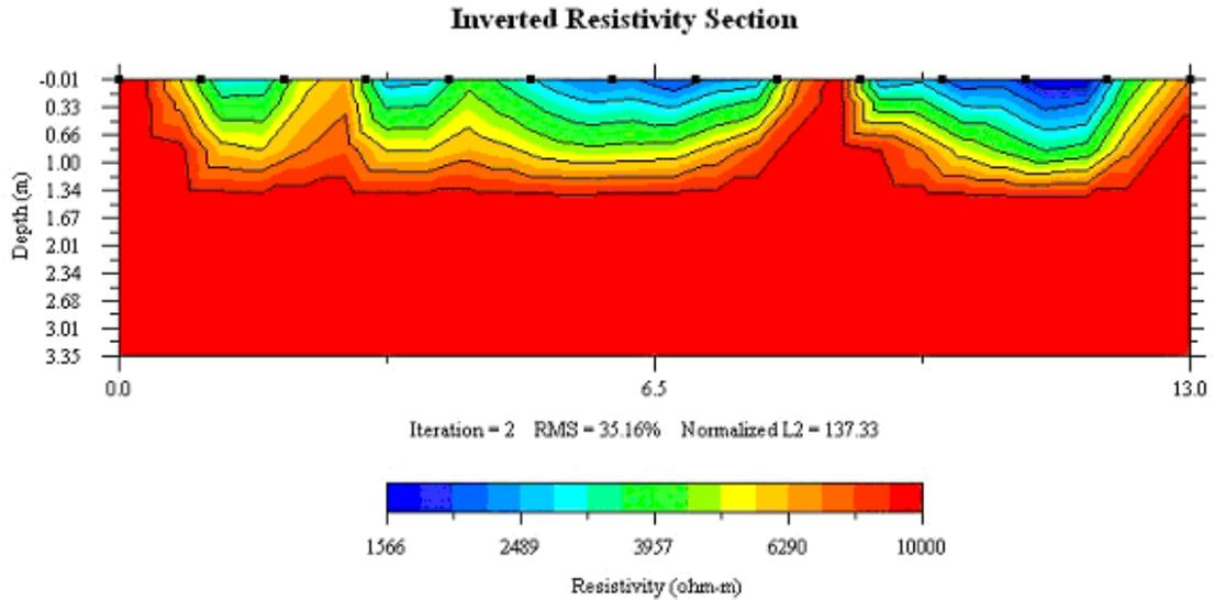
Fig. 1. Electrical Resistance cross-section from site 2 which is the debris field covering known glacial ice. The extremely high resistance can be anticipated, as glacial ice is an extremely poor conductor of electrical energy.
