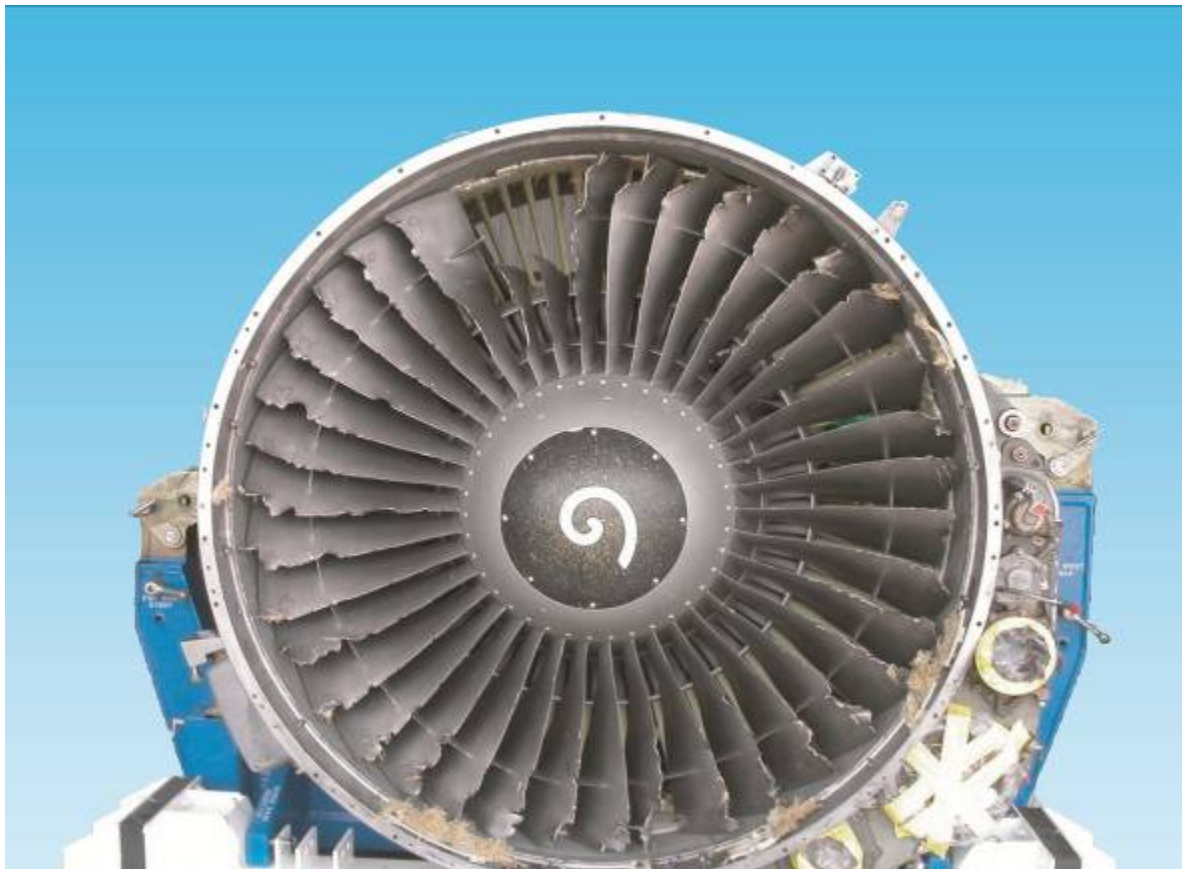
Fig. 4. An aircraft engine survived after a bird strikes in Central America. (Source: http://www.aviacrews.blogspot.com/ ).
