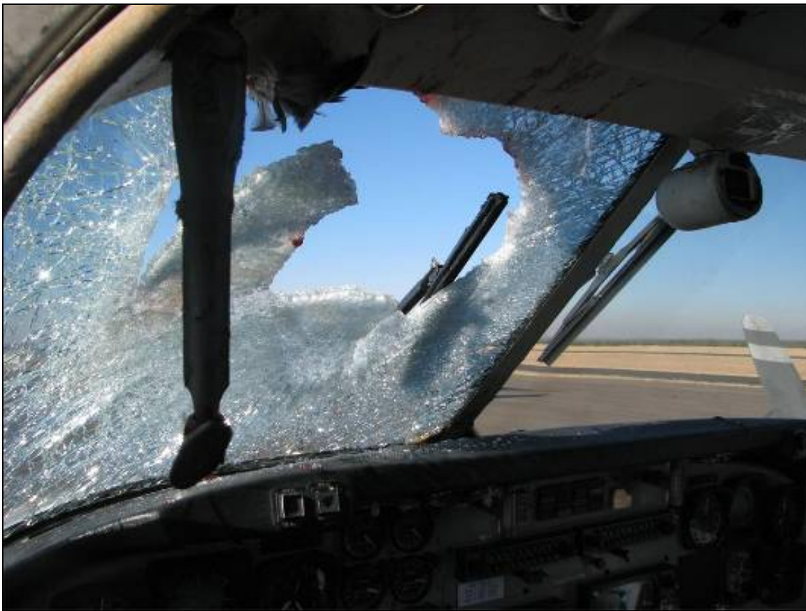
Fig. 2. Bird strikes cause damage of aircraft windscreen. (Source: http://www.birdstrikenews.com ).
