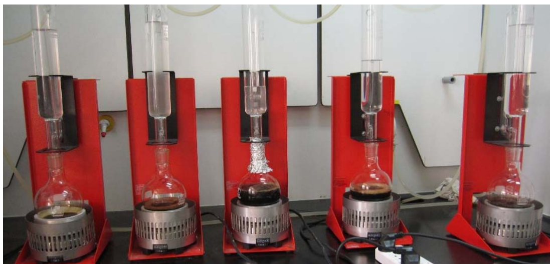
Fig. 1. Multiple Soxhlet Unit.
