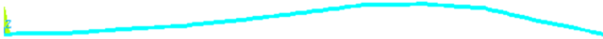
Fig. 9. The optimum design of a bent beam which minimizes the sound power level at over broad frequency band (exaggerated vertical scale).
