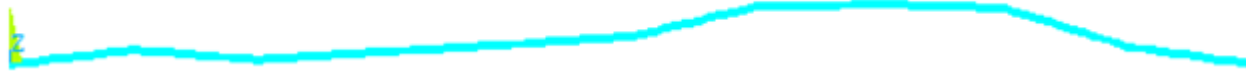
Fig. 7. The optimum design of a bent beam which minimizes the sound power level at 358 Hz (exaggerated vertical scale).
