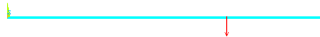
Fig. 4. The Optimum design of a bent beam which maximizes the gap between the fourth and fifth natural frequencies (exaggerated vertical scale).
