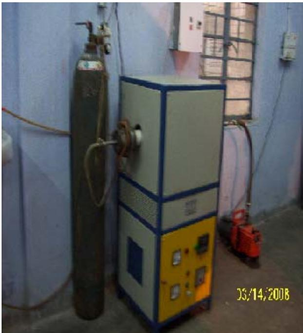
Fig. 11. Tubular vacuum furnace (1450°C).
