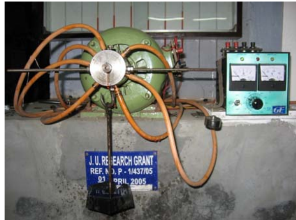
Fig. 3. Experimental set-up for measuring coefficient of friction of copper infiltrated P/M journal bearing.
