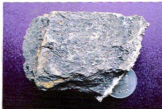
Fig. 3. Banded Hematite Quartzite sample, representing moderate grade Hematite ore. Near Vinukonda, Prakasam District.
