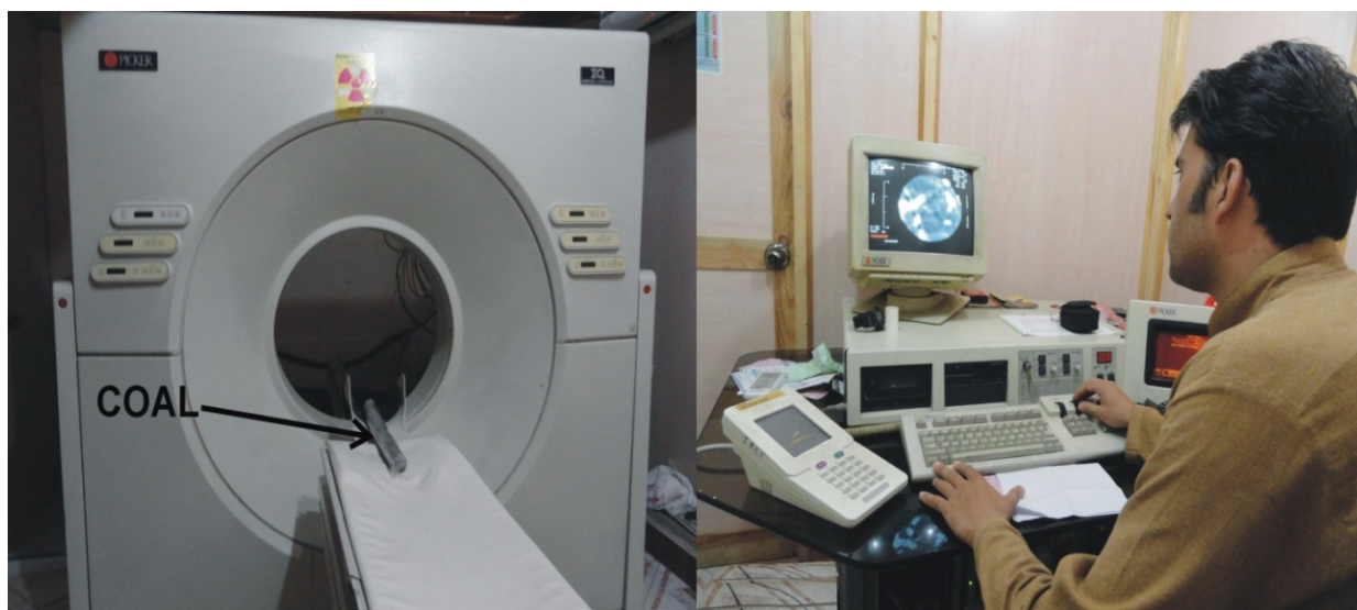
Fig. 2. Showing X-ray Computed Tomographic Scanning machine used in this study.
