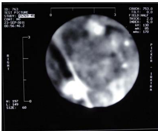
Fig. 6. X-ray view of slice, showing mineralization (pyritization) in cleats and pores.
